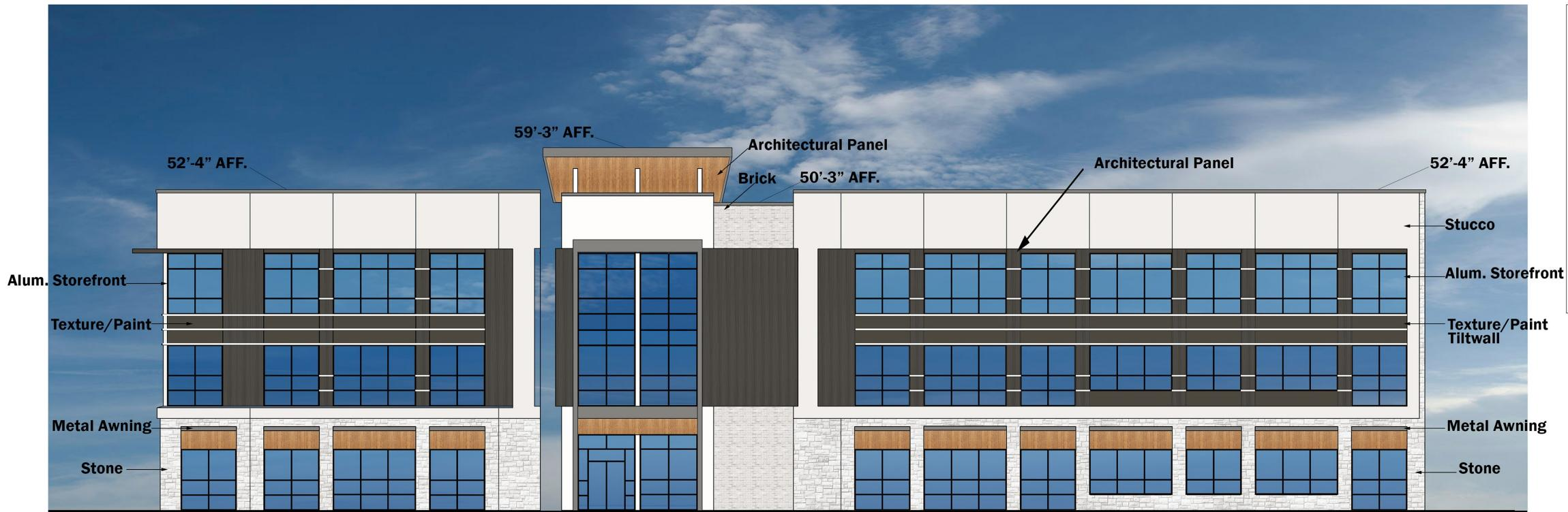
02a northeast elevation 02b northeast elevation
